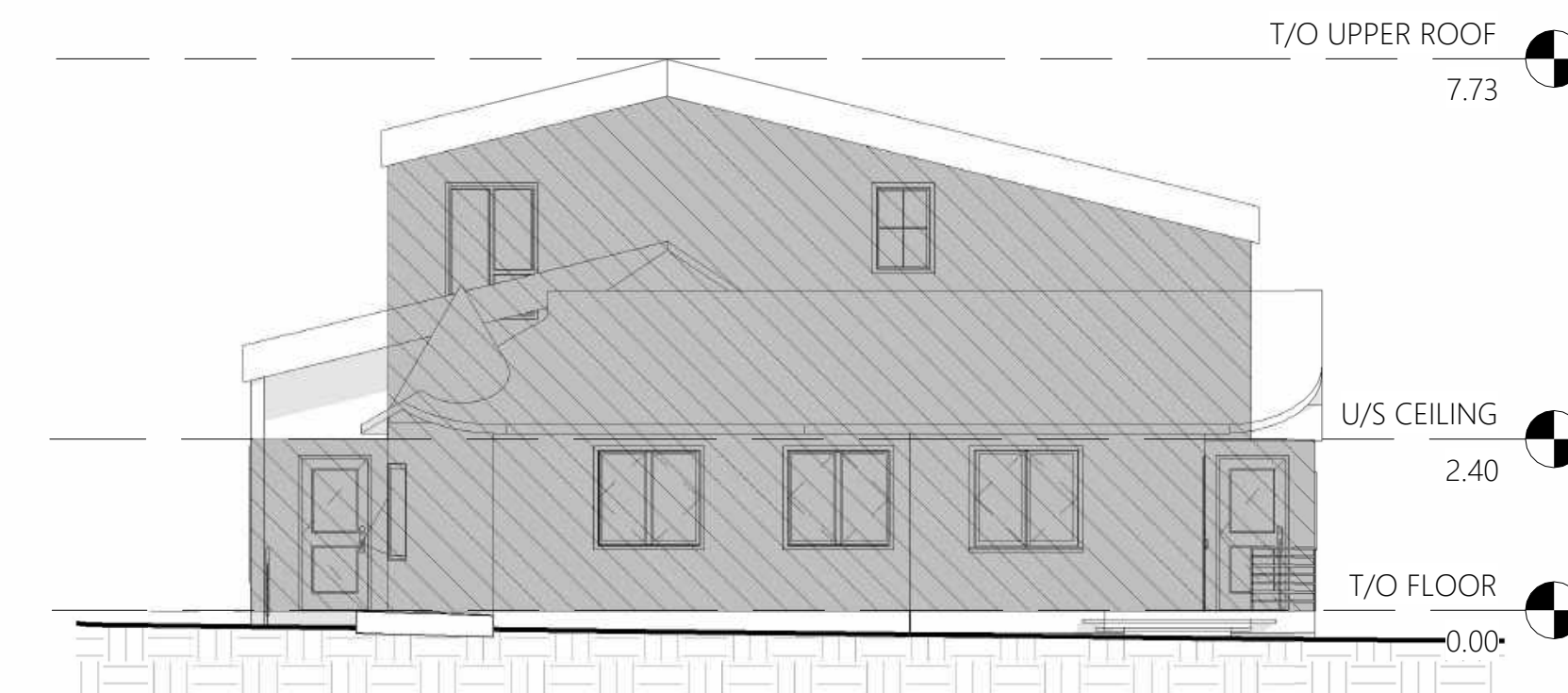
2 SOUTH ELEVATION UNPROTECTED OPENINGS 1: 100
