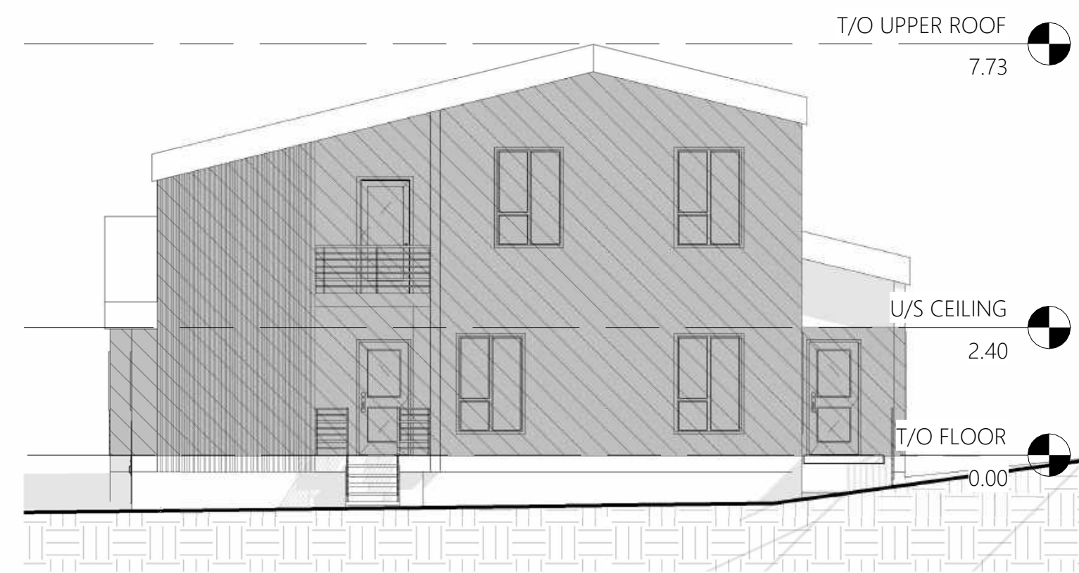
1 NORTH ELEVATION UNPROTECTED OPENINGS 1: 100
