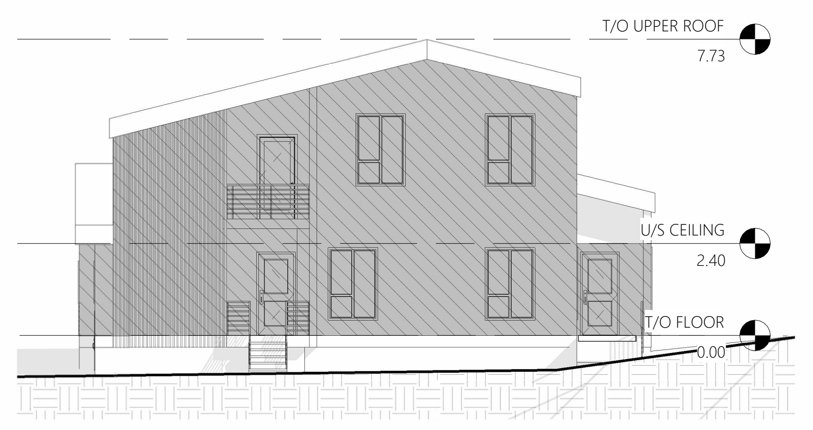
1 NORTH ELEVATION UNPROTECTED OPENINGS 1: 100
