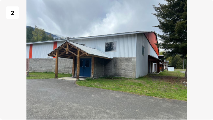
Main Entry 1. No paved walkway to access "accessible" ramp. Note, even with paved walkway, this ramp does not provide accessibility. See clarification further in report.
