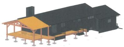
Review of the plans and an email from the applicant dated August 8, 2025, confirms that the new deck will be wood frame construction with concrete foundation piers and footings. The deck will be a self-supporting structure. The roof will be non-combustible.
